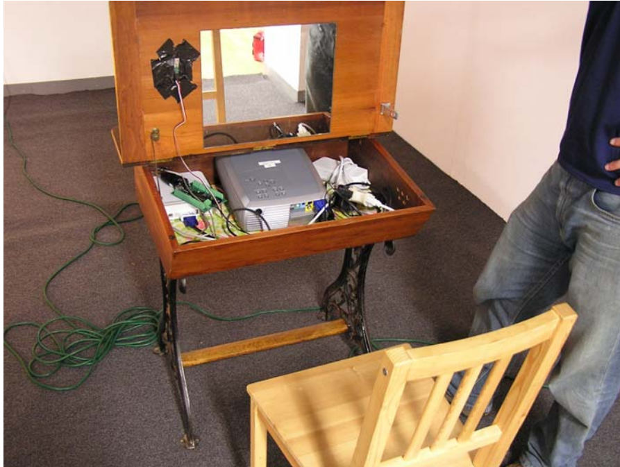
Educational Development, 2007. Inside of desk shows sensor, computer, projector. Final power supply solution will be concealed beneath carpet.
